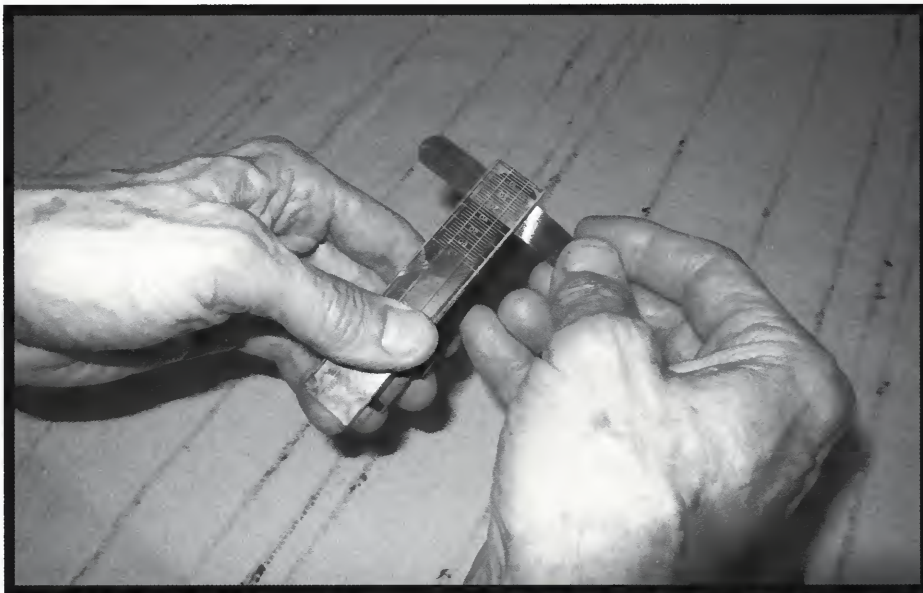
Mouthpiece facing curve being measured with Erick Brand glass and feeler gauge
